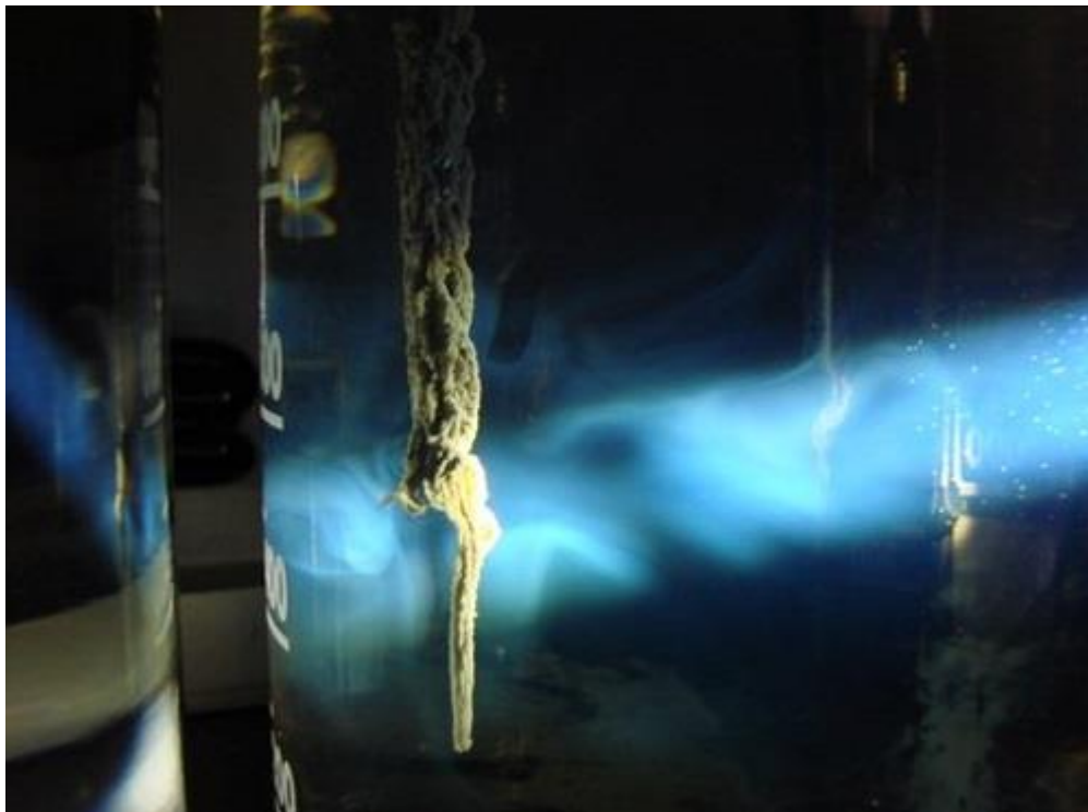
Figure 5. Illumination of water with silver nanoparticles using a white light source, showing colourful light scattering patterns. There is silver oxide present on the silver cathode.
