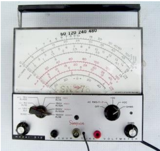
Figure 1. A typical vacuum tube voltmeter. The scale for resistance increases to the right and diminishes towards the left, which is opposite way to analogue multimeters. On this unit, the far right is a maximum value of 1,000 million Ohms.
