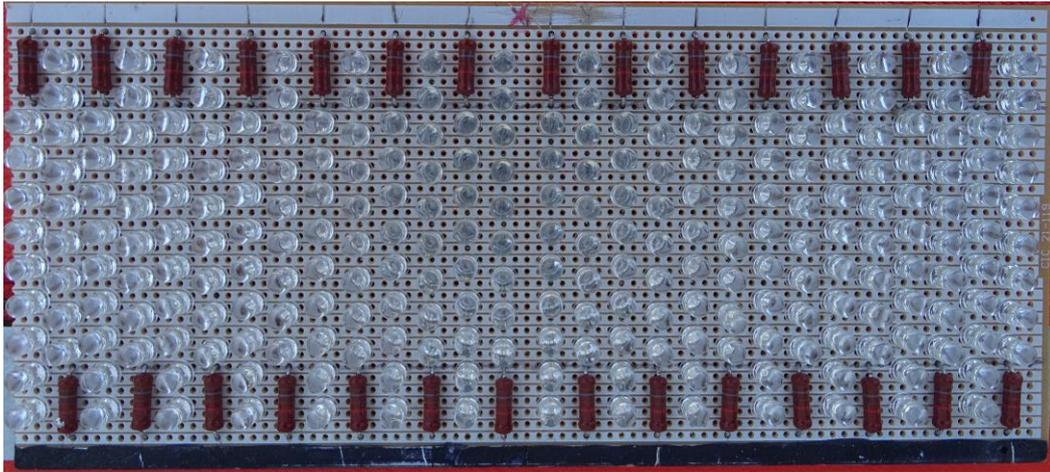
Matrix of 28 parallel rows of 9 violet LEDs wired in series making for 252 LEDs on an area of 250x100mm OCB. Instead of having rows of 10 at 3.5 volt =35 volt, columns of 9 allow for 4 volt per LED = 36 volts in total and within the limit set by the LM317T voltage regulator.
